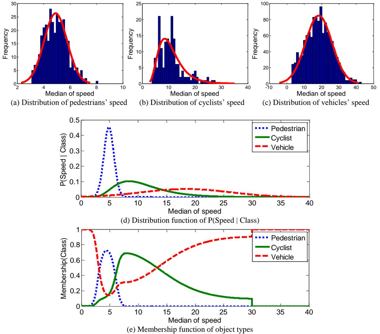
Figure 4. Speed distribution and membership function of each object type used for classifier's design
