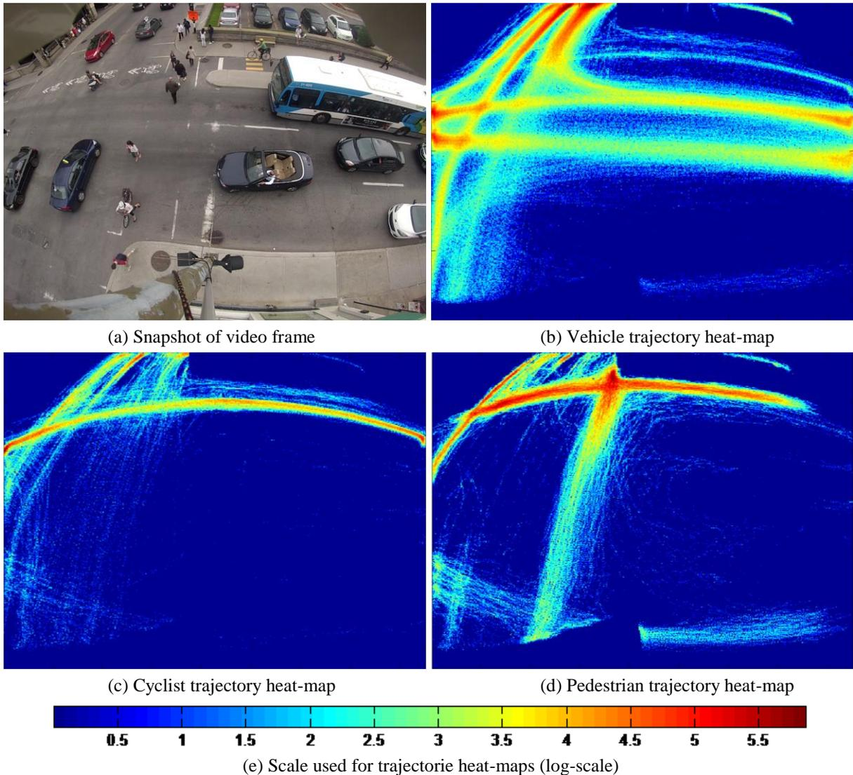
14 Figure 6. Snapshot of video and position heat-maps for the three road user types (taken from Classifier V). The most
