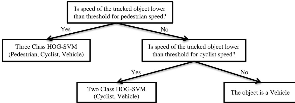
Figure 3. Flowchart showing the use of speed thresholds to switch between classifiers
