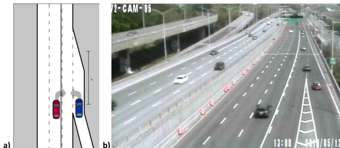
Figure 4 – LCGV1. a) Exit ramp section diagram demonstrating an LCGV1 and an illegal lane change. Lanes are numbered sequentially starting with the outer-most lane, excluding merging lanes. b) LCGV1 along autoroute 720 eastbound, entrance 3 (right), Montreal. Source: MTQ.
