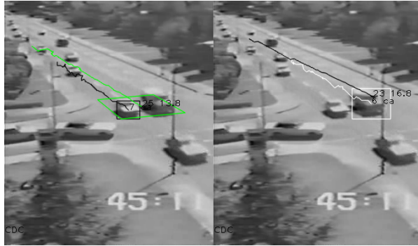
Figure 1: Example of two correct object assignments, ground truth object 7 to detected object 25 on the left, ground truth object 6 to detected object 23 on the right. In this typical case of close objects with consistent motion, a simple unique assignment may first assign the ground truth object 6 to the detected object 25, in which case it is very likely that the ground truth object 7 will not be assigned to the detected object 23, which will count respectively as one missed detection and one false detection.
