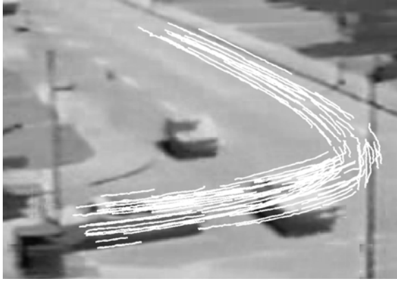
FIGURE 2 Example of disrupted feature tracks that are still successfully grouped.
