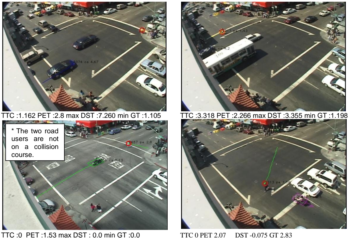
Figure 4 - Sample frames with automated road user tracks. The captions display “Event” the event order in the list of potential interactions, “objects” the numbers of the interacting objects, and the indicated conflict indicators.
