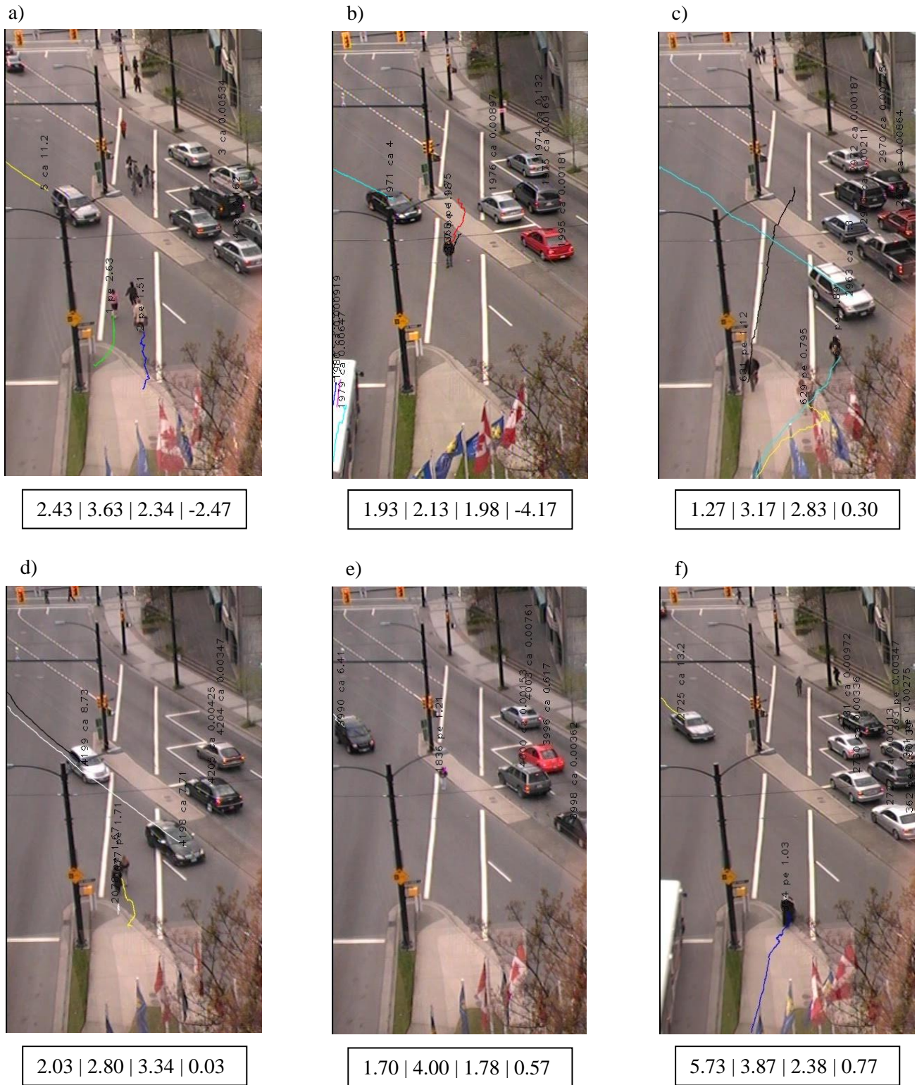
FIGURE 5 Sample of automatically detected important events with the road users' trajectories. The numbers under each image are respectively the min TTC (seconds), PET (seconds), maximum DST ( m/s^2 ), and min GT (s). In the images, the road user speed is indicated in m/s.
