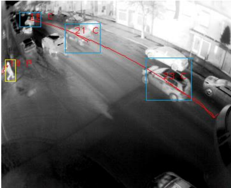
10 FIGURE 6 Tracking & Classification process with video - Sample of tracking and 11 classification. The red line represents the trajectories of the moving objects up to the time 12 of the image; P stands for pedestrians and C stands for cars
