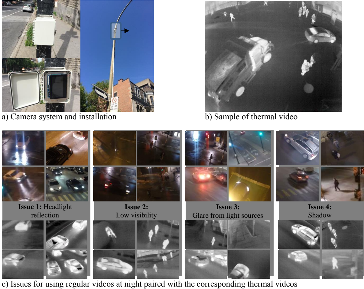
10 11 12 13 14 15 16 17 18 19 20 21 22 23 FIGURE 1 Thermal camera system and a comparison with regular videos at nighttime
